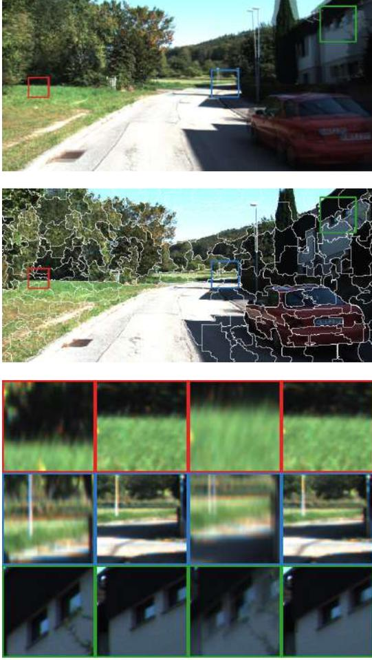
Fig. 3: Comparison of different alignment methods. Top: the alignment result from global homography transform; mid: superpixel segmentation for sample input; bottom: local detail comparison on three selected positions. While the first two columns are source and target patches, the last two columns are alignment results from homography-based method and superpixel-based method.
